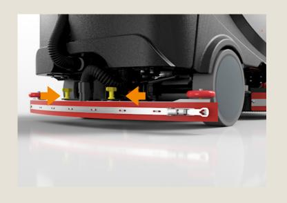
Install the squeegee and attach it by using the two knobs.
