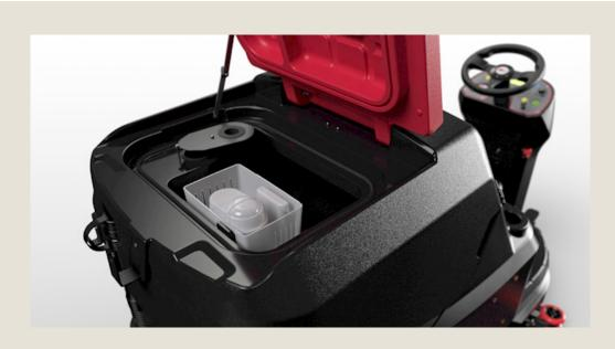
Park the machine leaving the recovery tank open.
