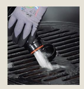
Empty the tank with the hose in the back. Empty and clean the debris tray in the tank, flush&clean out the recovery tank.
