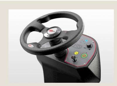
During the cleaning job it's possible to adjust the solution flow, the brush pressure, activiting Eco Mode or Silent Mode from the dashboard.
