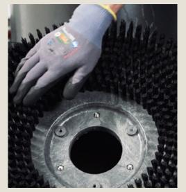
With the key turned on press the brush click off button to remove the brushes/pad holders for inspection and cleaning.
