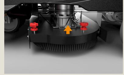
To install the brush/pad holder, pull up the metal handle and slide in the brush/pad holder until it stops against the pins in the proper position and release the handle. Reinstall the side skirt.
