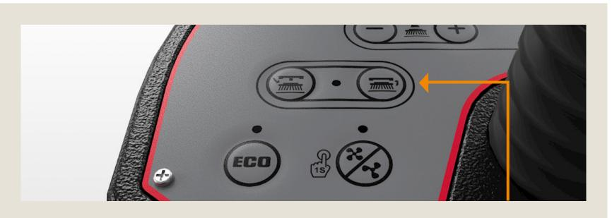
Turn the main key to on and press the click on button to install the brush automatically. Deck will lower and brushes turn slowly to attach.
