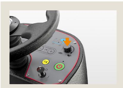
Adjust the maximum speed with the speed adjustment dial.
